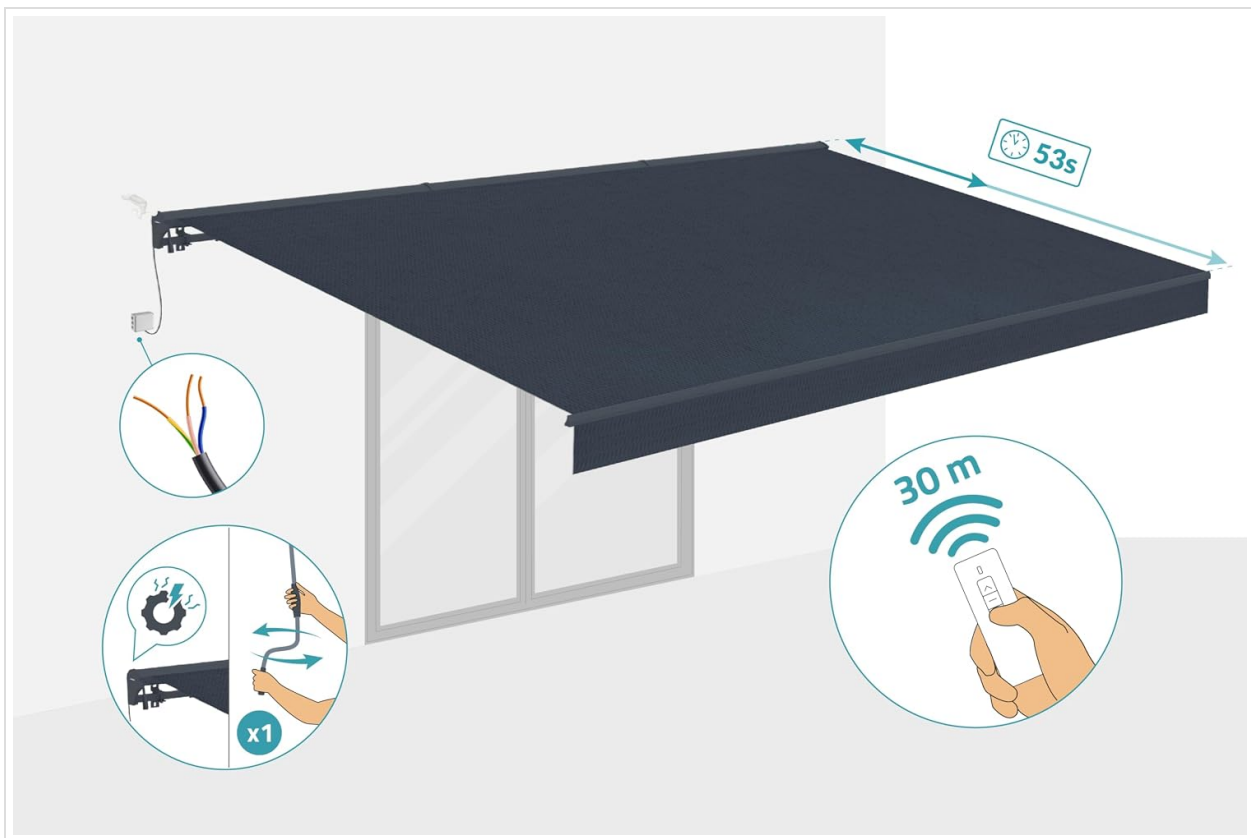
Image 5.1: This image shows the remote control with a 30-meter range and the manual crank handle for emergency operation. It also indicates an approximate extension/retraction time of 53 seconds.
