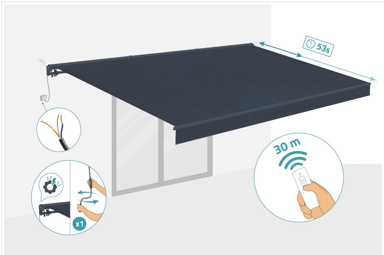
Image 4.3: Illustration detailing the electrical wiring connection for the awning motor and the remote control's operational range.
