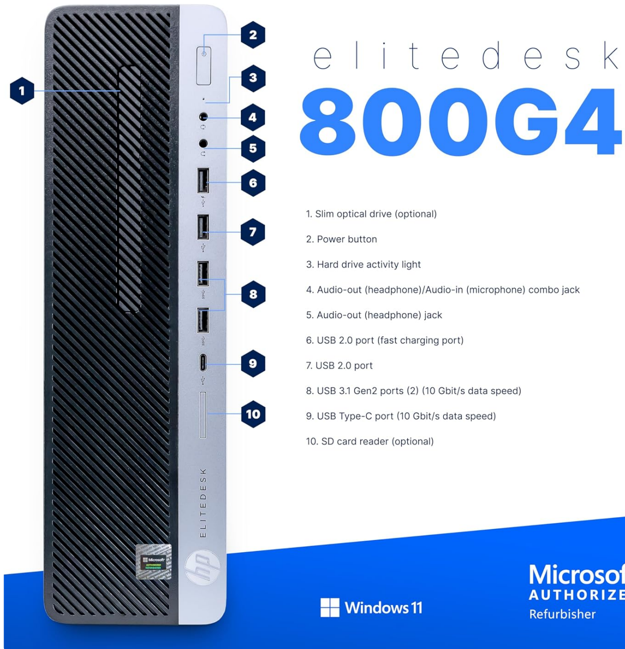
Image 2.2: Front view of the HP EliteDesk 800G4 PC, illustrating USB 2.0 ports (labeled 6, 7), USB 3.1 Gen 2 ports (labeled 8), and a USB Type-C port (labeled 9).
