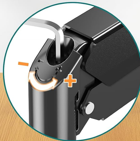
Figure 5: Tension adjustment. This image provides instructions on how to adjust the gas spring tension using an Allen key. Turn clockwise ("-") if the arm rises, and counter-clockwise ("+") if the arm falls, to match your monitor's weight.
