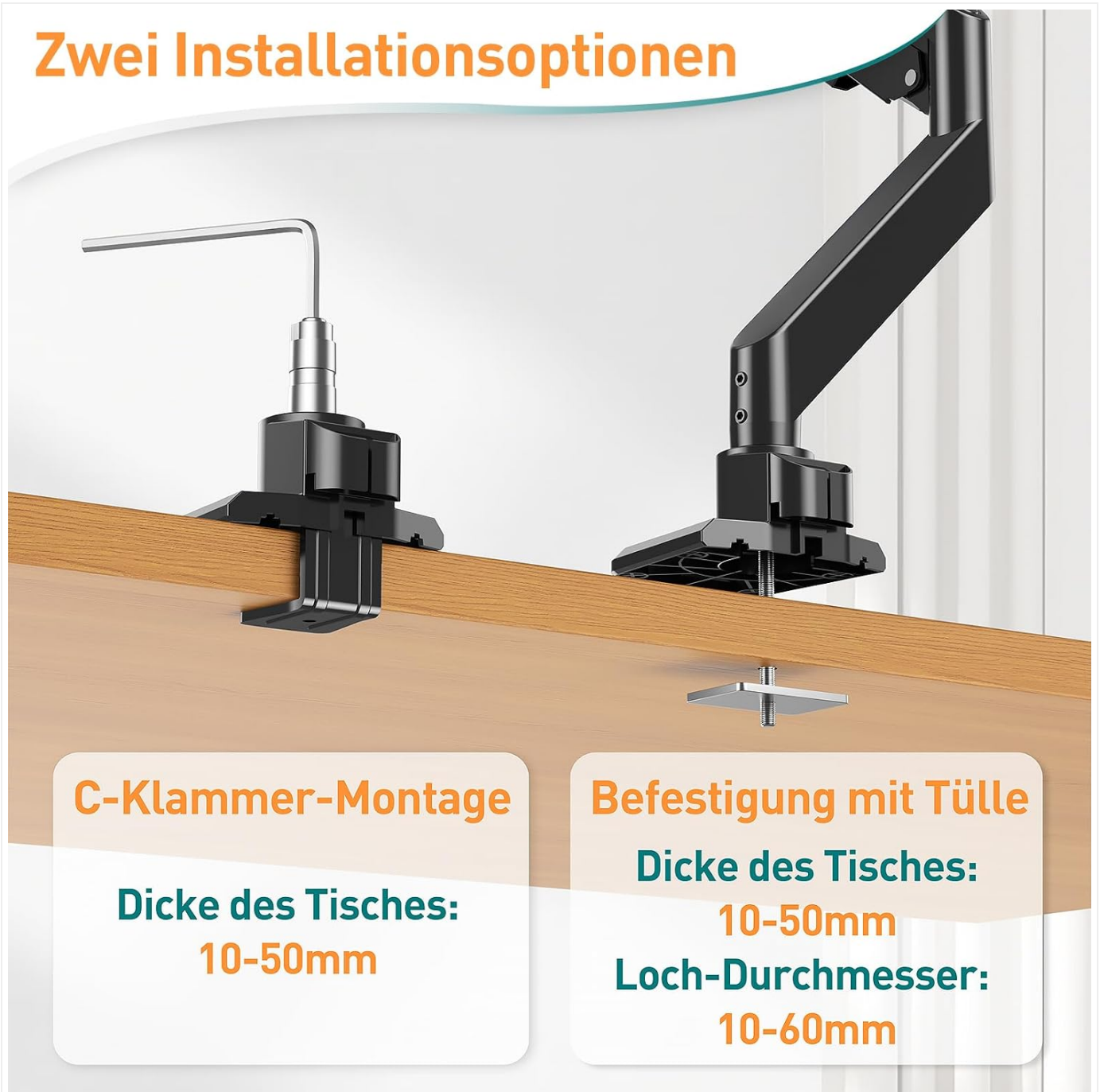
Figure 2: Two installation options. The image displays both the C-clamp and grommet mounting methods, detailing the required desk thickness (10-50mm for both) and hole diameter (10-60mm for grommet mounting).
