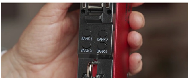
Figure 4.7: The LCD display and bank buttons for quick access to settings.
