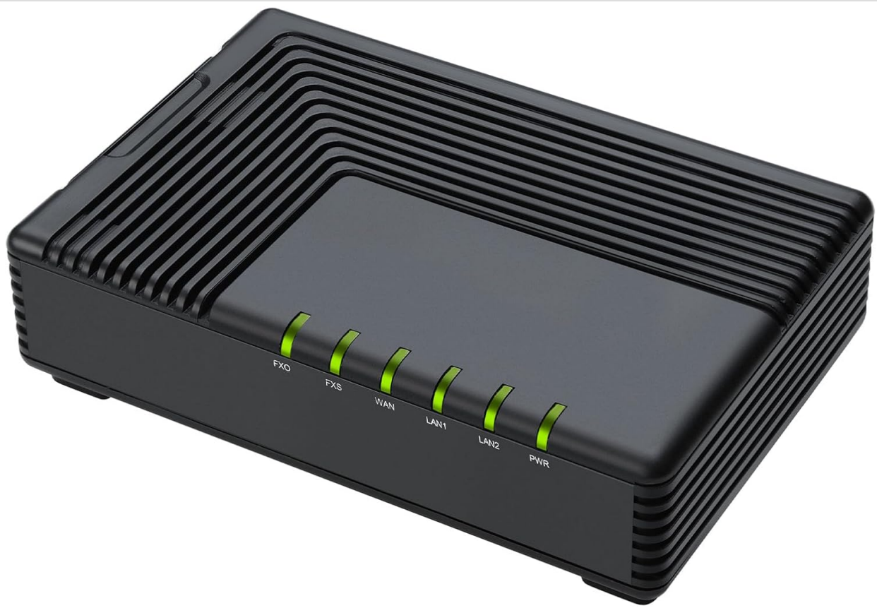
Image: Front panel of the FTA5111 with LED status indicators.
