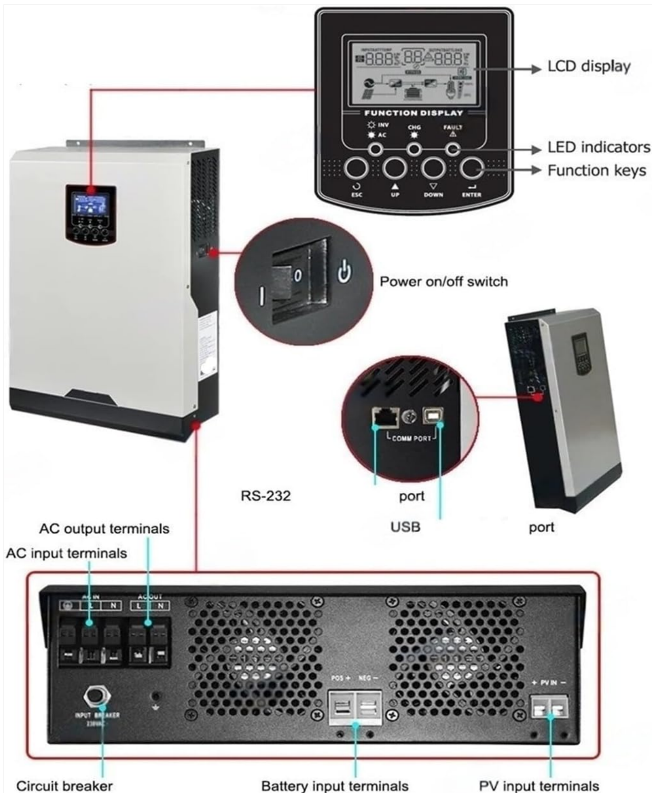
Figure 3.1: Front and rear panel components of the inverter.
