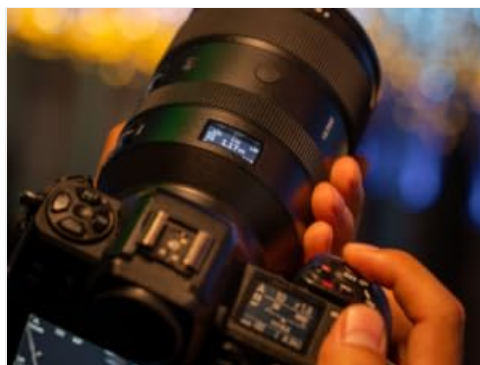
Figure 6: Detail of the AF/MF switch and one of the customizable focus hold buttons.
