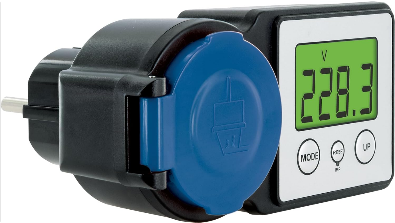
Image: The energy cost meter's display showing a voltage reading of 228.3 V, demonstrating one of its measurement modes.
