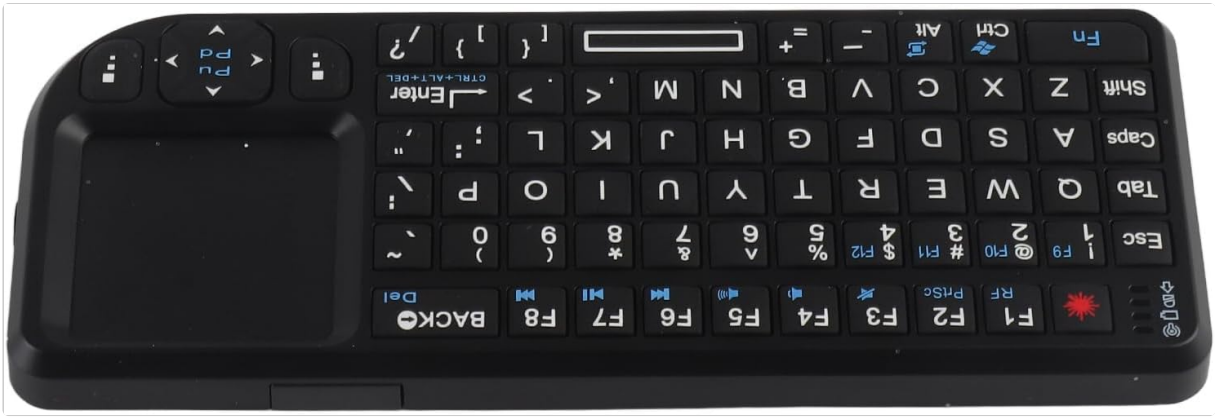
Figure 1: Top view of the Yoidesu Mini Bluetooth Keyboard, showing the QWERTY key layout, touchpad on the left, and navigation buttons.
