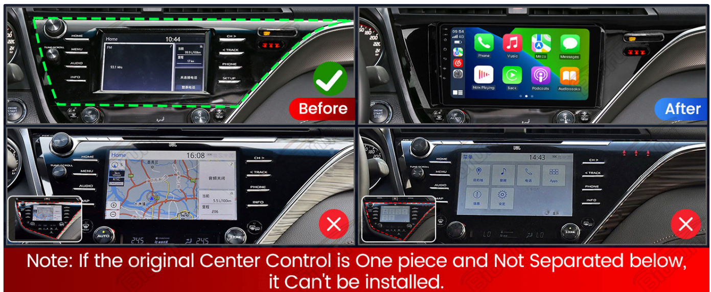
Image 2.1: Visual guide for checking car radio compatibility with Toyota Camry center console. The top image shows a compatible separated console, while the bottom images show incompatible one-piece consoles.
