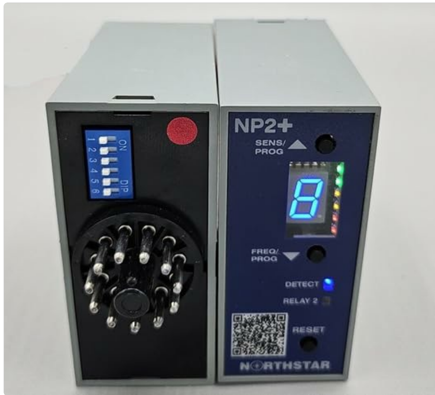
Figure 1: Northstar NP2+ Loop Detector. The left unit shows the 6-position DIP switch and multi-pin connector. The right unit displays the 'NP2+' model name, 'SENS/PROG' and 'FREQ/PROG' buttons, a digital display showing '8', and 'DETECT' and 'RELAY 2' LED indicators. A 'RESET' button and 'NORTHSTAR' branding are also visible.
