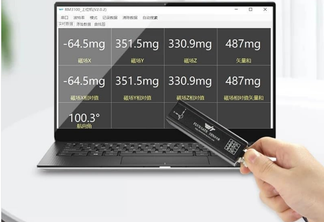
Figure 3: PC Software Interface. This image shows a laptop screen displaying the RM3100 Host Computer Software, which visualizes three-axis magnetic field data (X, Y, Z) in milligauss (mg) and the calculated heading angle (100.3°). The sensor is shown connected to the laptop.
