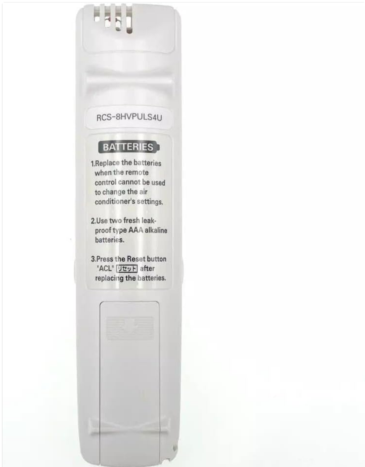
Image: Back of the remote control, illustrating the battery compartment and battery replacement instructions.
