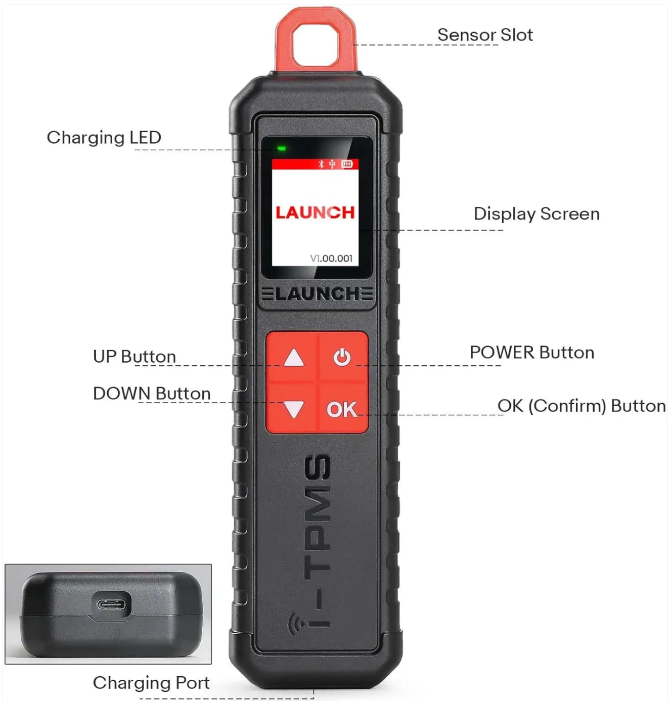
Figure 2.2: Labeled components of the X-431 i-TPMS device.
