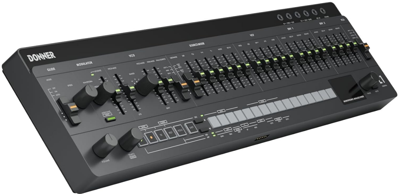
Figure 1: Front view of the Donner ESSENTIAL L1 Synthesizer, showcasing its control panel and compact design.
