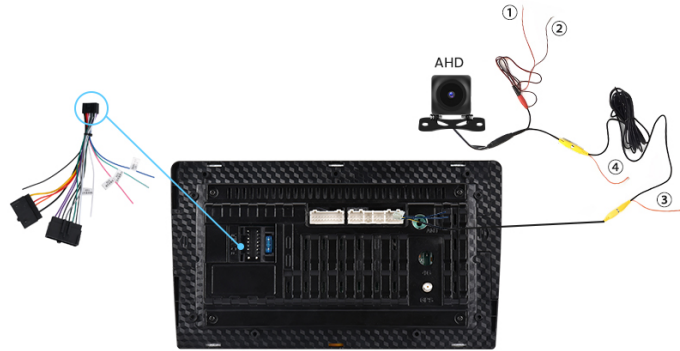
Figure 4.2: Detailed wiring diagram for the reversing camera.
