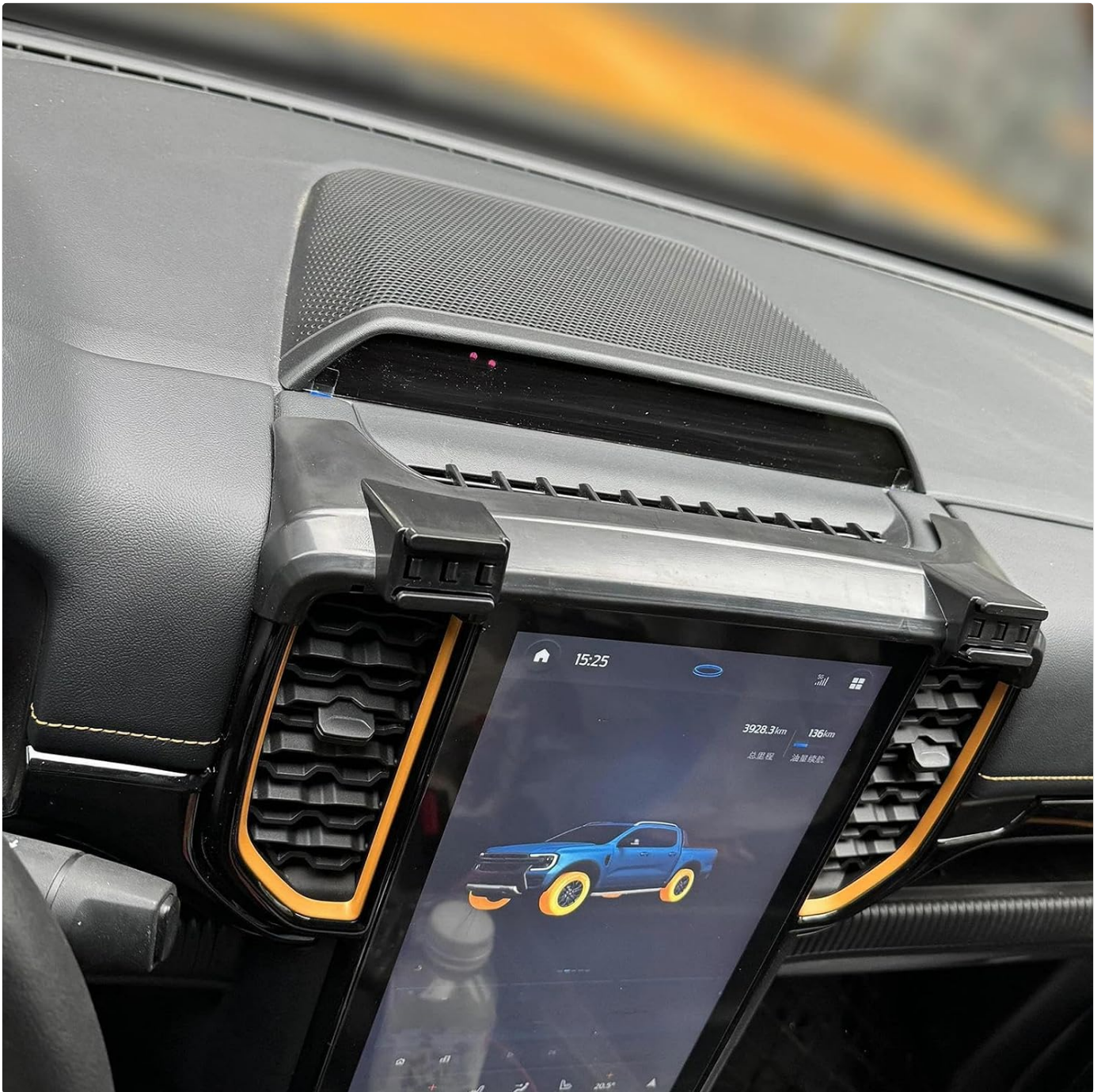
Figure 2.2: Example of the base installed on the vehicle dashboard.
