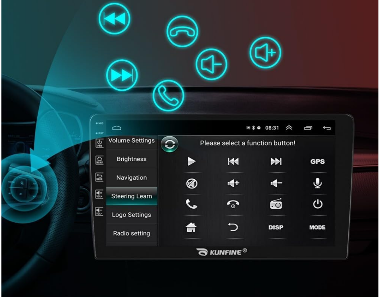
Image 4.7: The interface for configuring steering wheel controls, showing various assignable functions.
