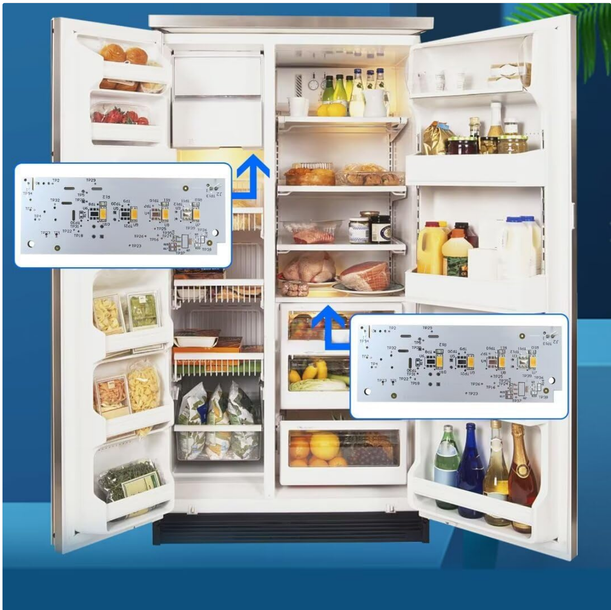
Figure 5.2: A visual representation of where the LED light boards are typically positioned inside a refrigerator, indicated by blue arrows.
