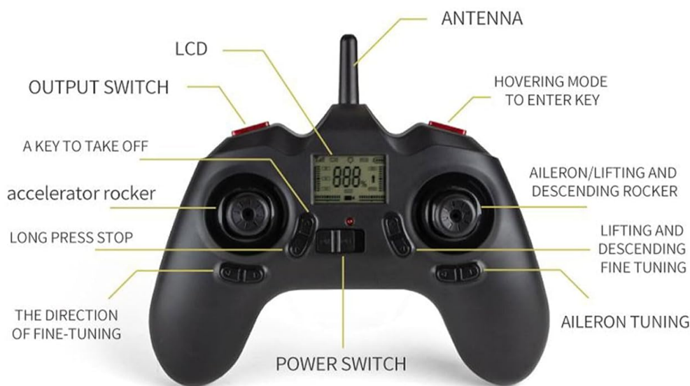
Image: Diagram of the remote control, highlighting its various buttons and sticks, including the LCD display and antenna.
