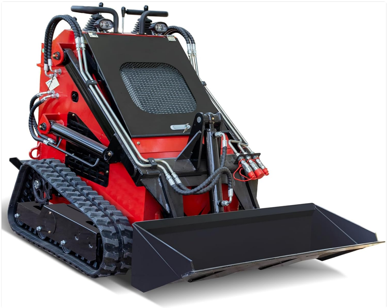
Figure 1: MMS Mini Triangular Track Skid Steer Loader (Model MS380T) with 46-inch bucket.
