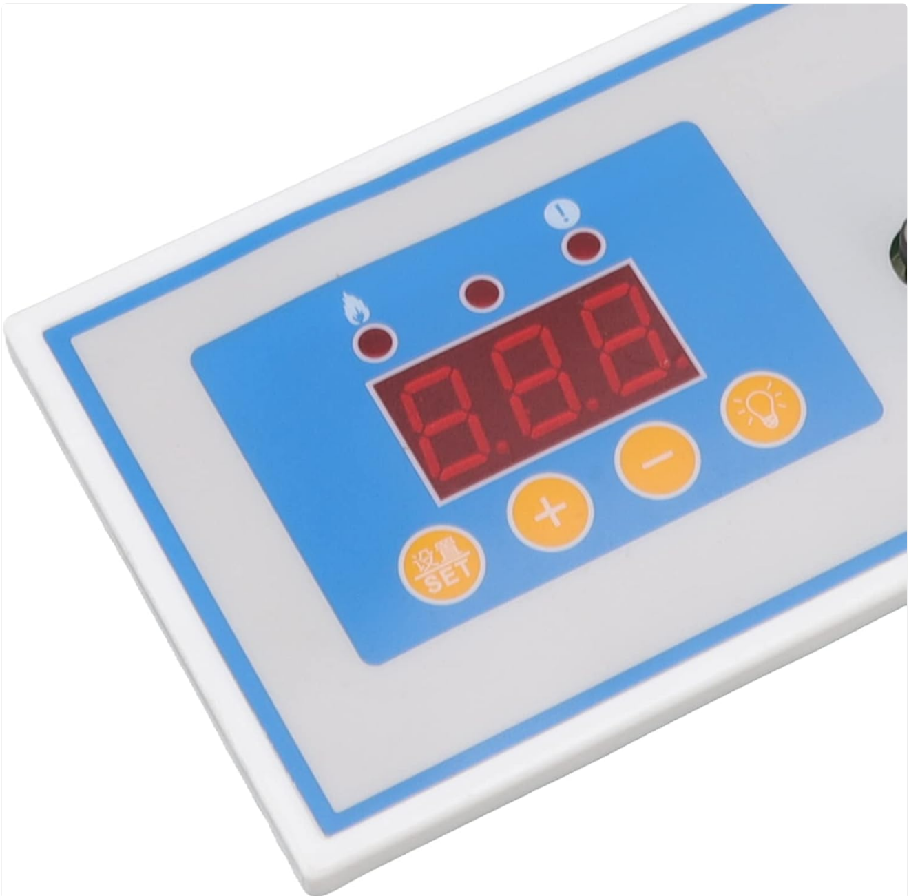
Image 3.1: Close-up view of the control panel, showing the digital display, SET button, plus (+) button, minus (-) button, and light button.
