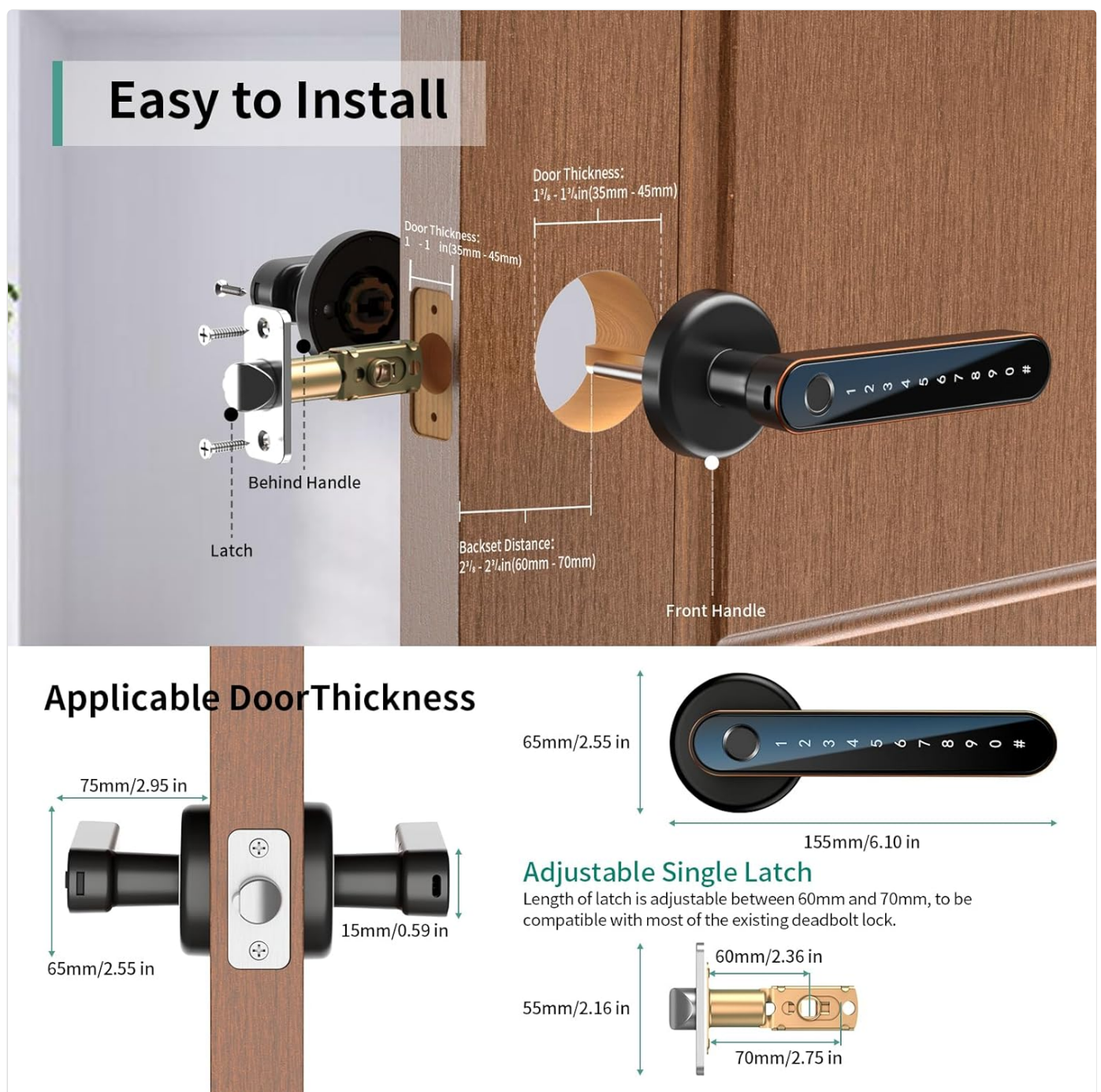
Image: A detailed diagram illustrating the installation process of the IRONZON Fingerprint Door Lock, including measurements for
