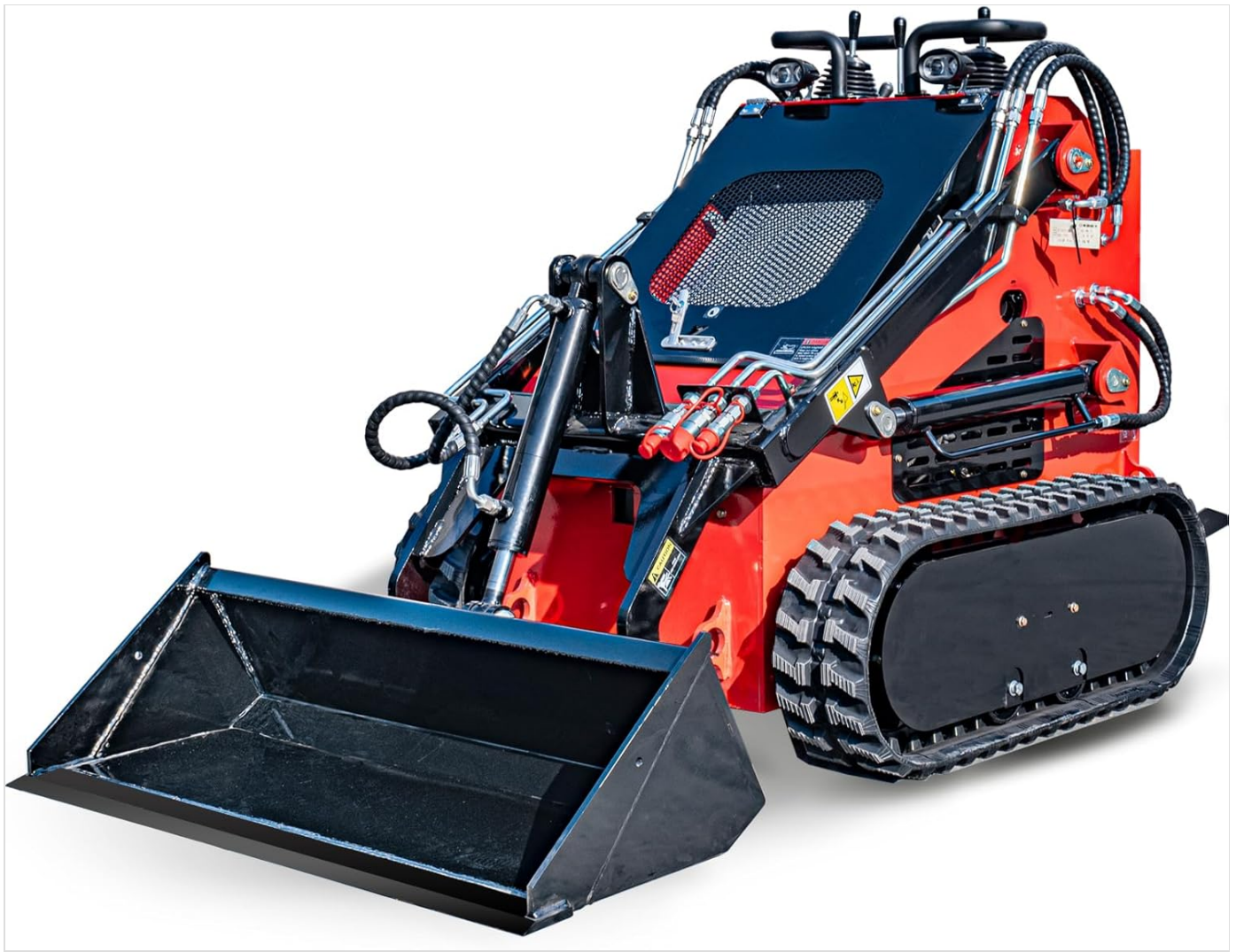
Figure 3.2: The MMS MS380-C Mini Skid Steer Loader with its standard front end bucket attached, ready for operation.
