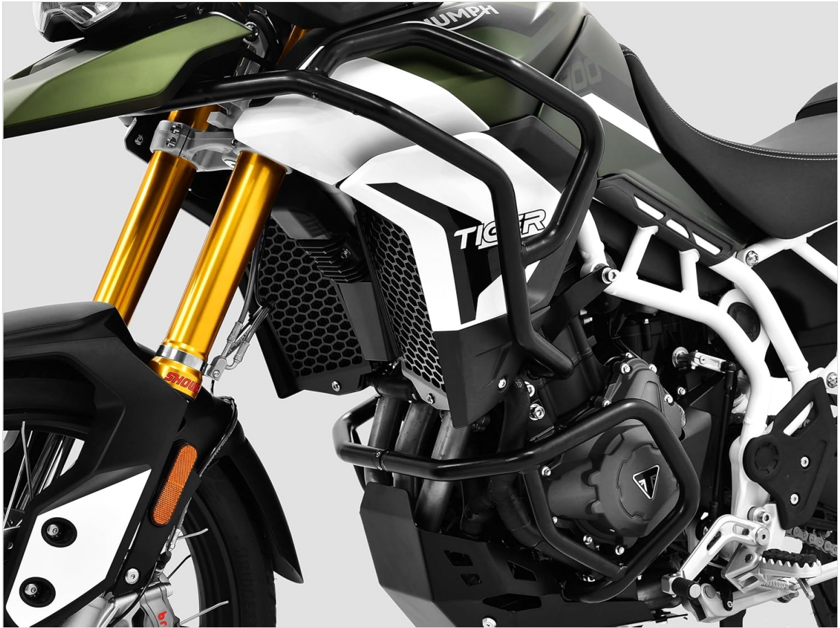
Figure 1: Frontal view of the ZIEGER crash bar installed on a Triumph Tiger 900. This image highlights the robust construction and how the bar integrates with the motorcycle's frame, providing protection to the engine and radiator area. Note the secure mounting points visible around the engine casing and lower frame.
