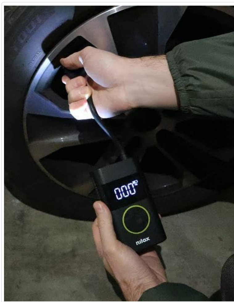
Image: A person holding the Nilox Mini Portable Air Compressor, which displays '000', while the attached hose is connected to a car tire valve for inflation. The integrated LED light is active.
