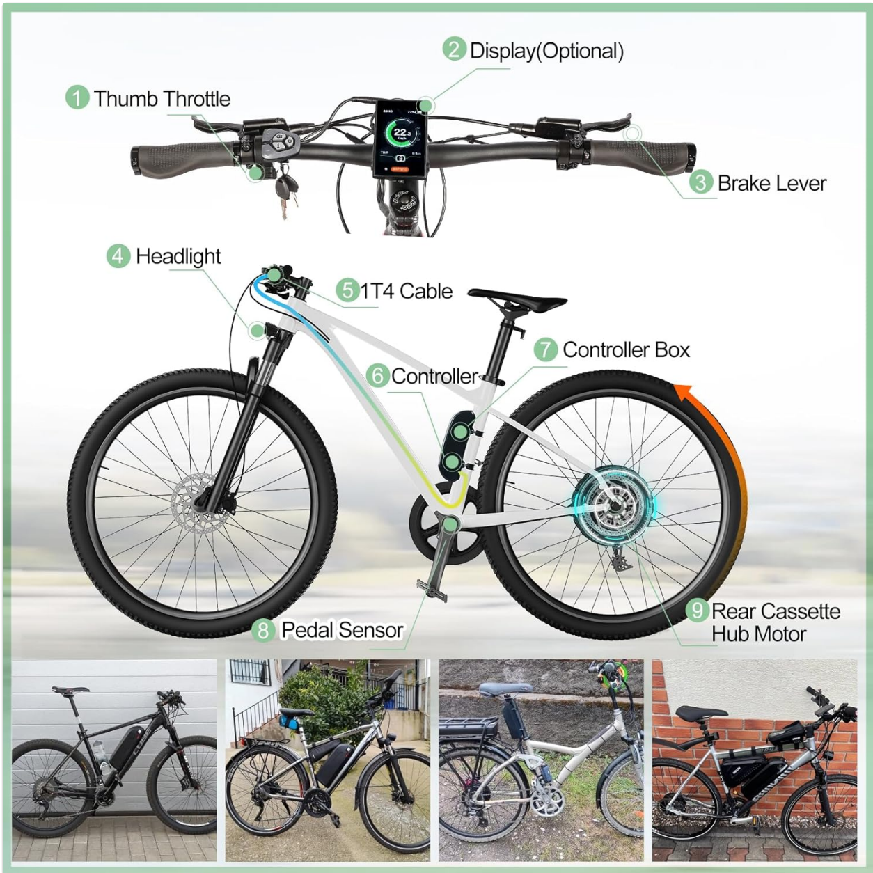
Image 2.2: Component Diagram. This diagram illustrates where each component of the conversion kit is typically installed on a bicycle frame, including the thumb throttle, display, brake lever, headlight, 1T4 cable, controller, controller box, pedal sensor, and rear cassette hub motor.
