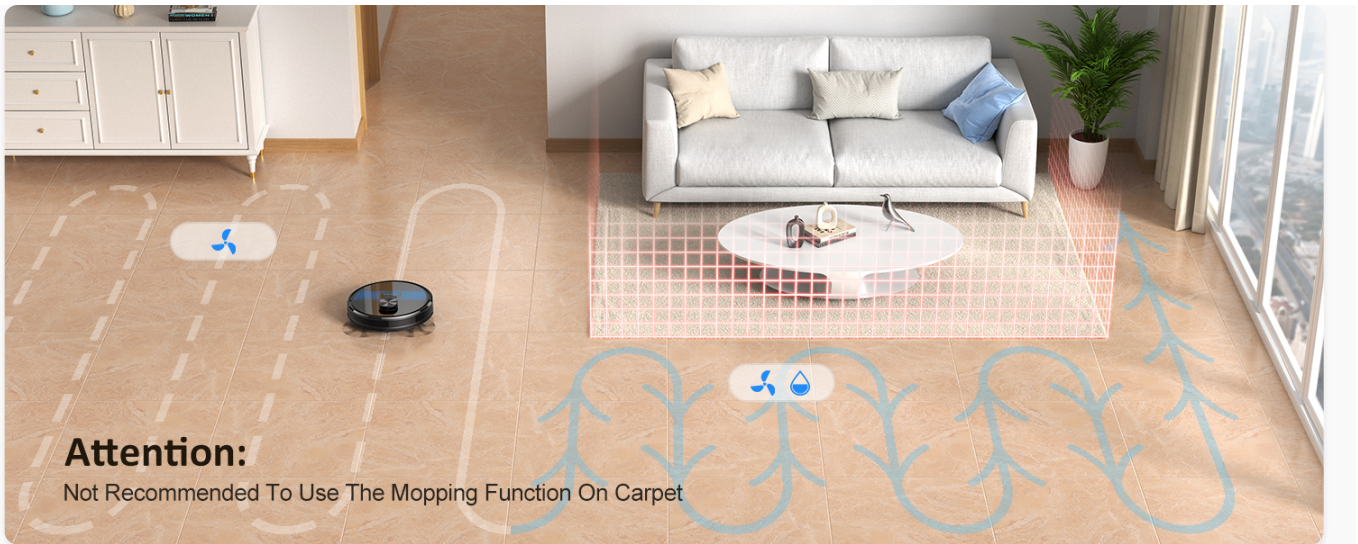
Image: An illustration showing the Lubluelu SL60D robot vacuum performing assigned area cleaning and spot cleaning within a house layout, controlled via a mobile app.
