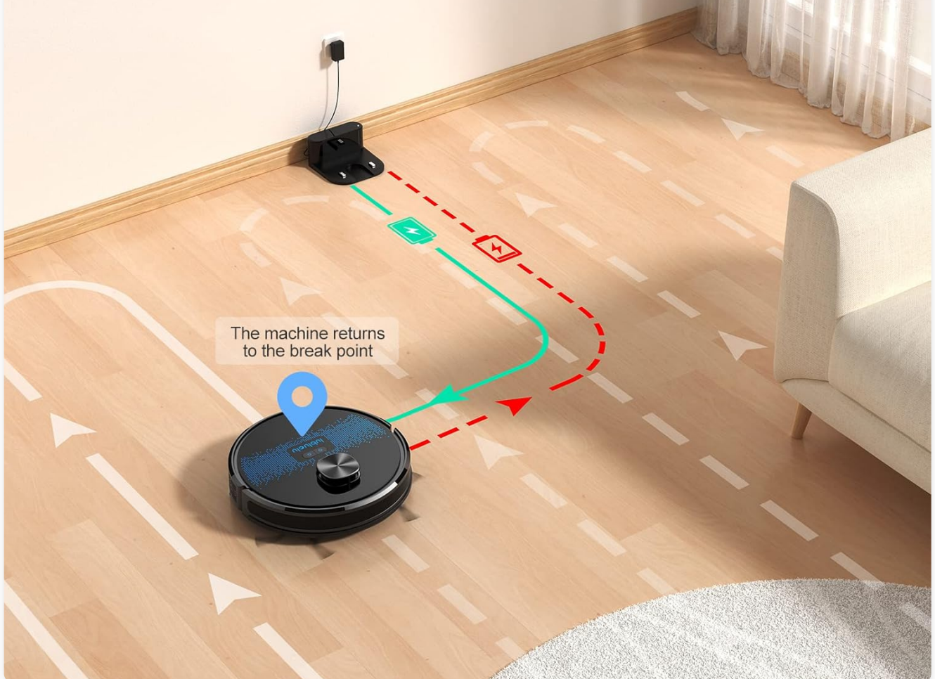
Image: A diagram showing the Lubluelu SL60D robot vacuum returning to its charging dock when the battery is low and then resuming cleaning from the breakpoint.
