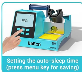
Figure 6.2: The sleep mode feature automatically lowers the iron's temperature when idle, and auto-wakes when picked up.
