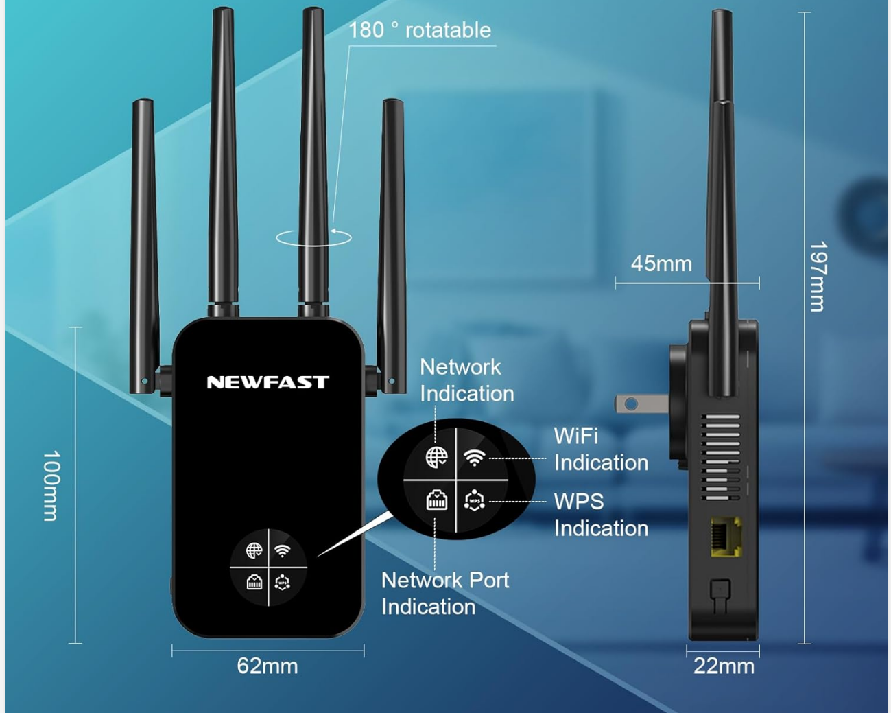
Image: Detailed view of the WiFi repeater's smart LCD display and physical dimensions, showing network, WiFi, and WPS indicators.
