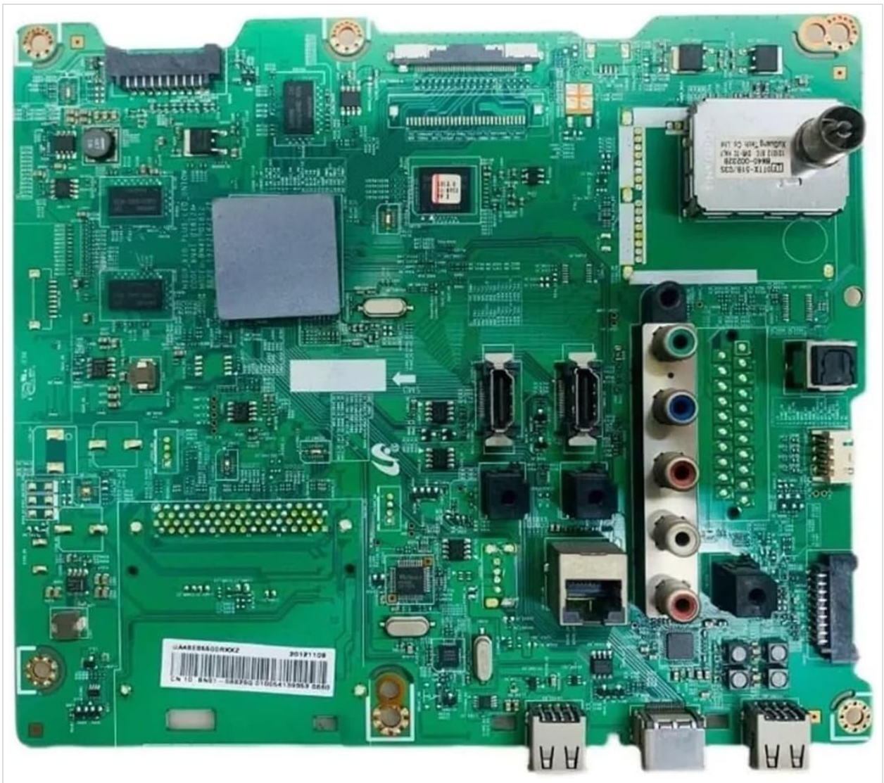
Image 2.1: Front view of the CFguang BN41-01812A TV Main Board, showing various ports and components.
