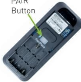
Figure 5: Pairing instructions for older Ease models, highlighting the Battery Backup Box and remote PAIR button.
