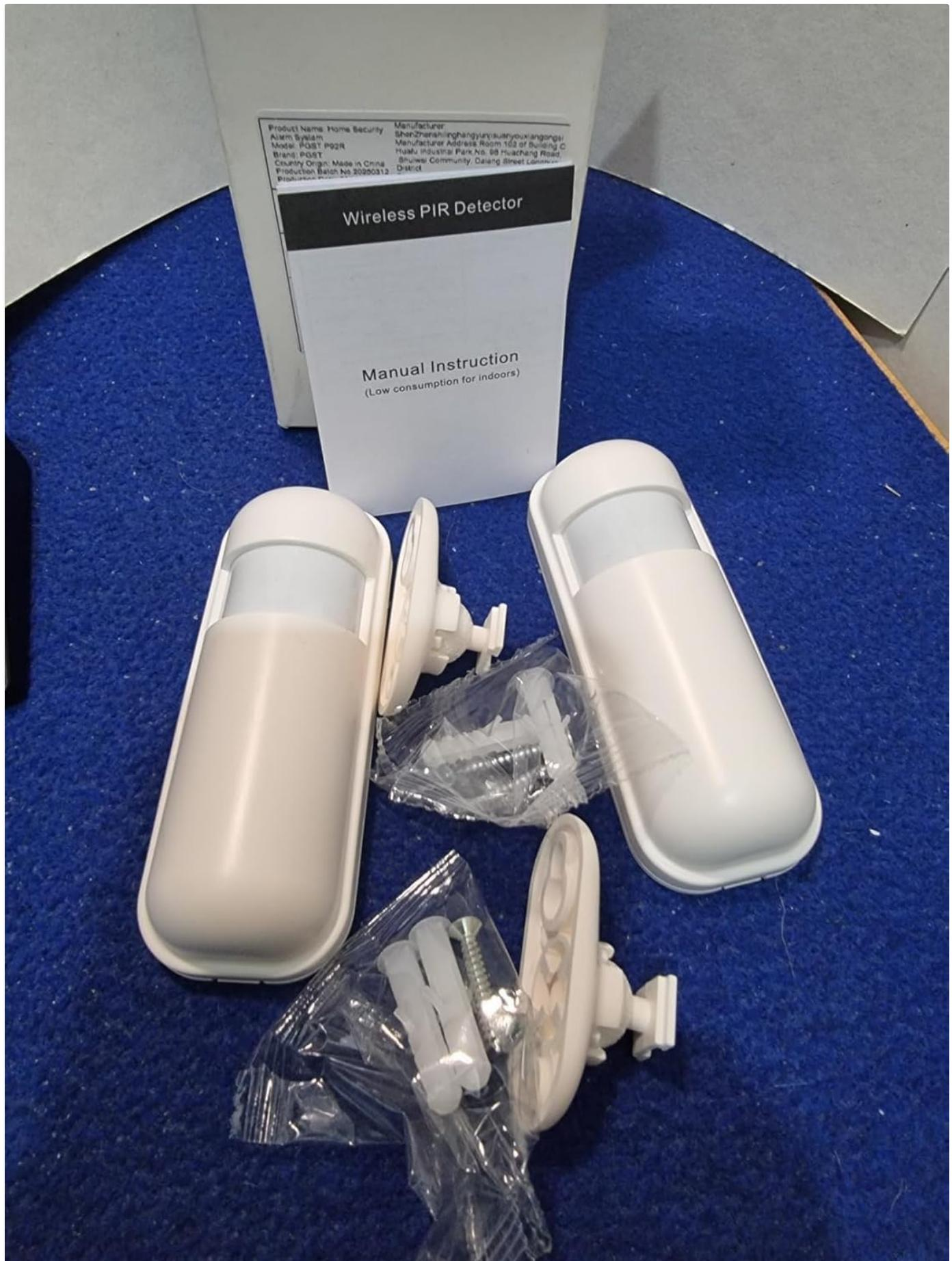
The PGST P92R-3 sensor is displayed alongside its mounting accessories, including screws and wall anchors, ready for installation.
