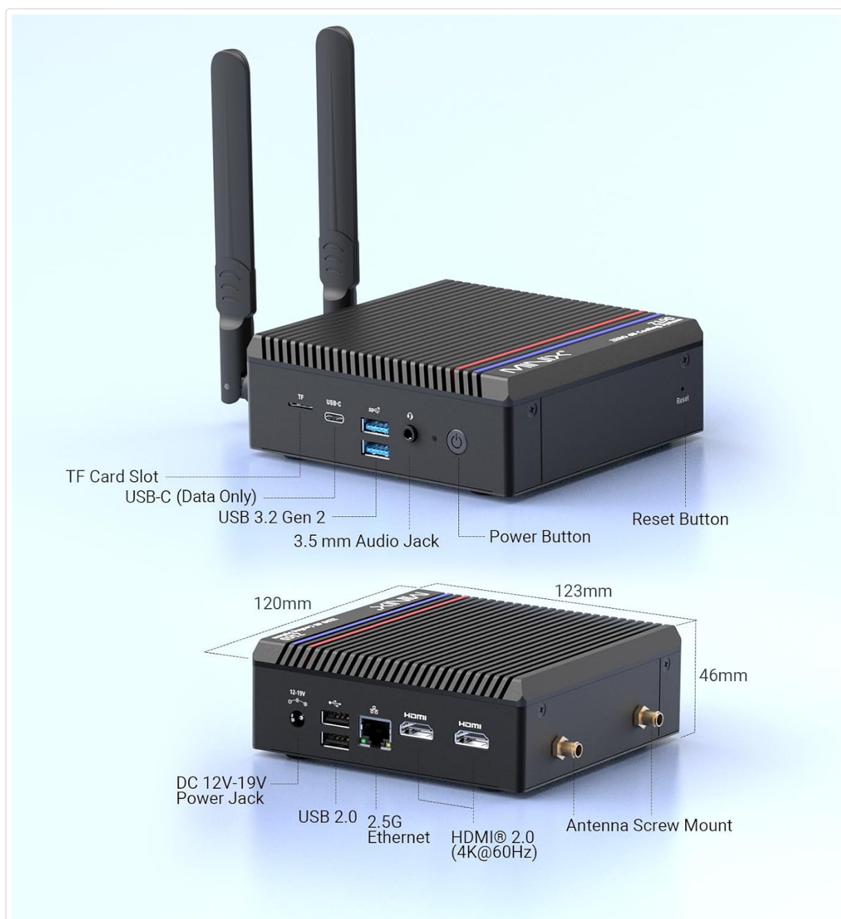
Image 4.1: Detailed diagram showing the port layout and dimensions of the MINIX Z150-0dB Mini PC, including TF Card Slot, USB-C (Data Only), USB 3.2 Gen 2, 3.5 mm Audio Jack, Power Button, Reset Button, DC 12V-19V Power Jack, USB 2.0, 2.5G Ethernet, HDMI 2.0, and Antenna Screw Mounts.
