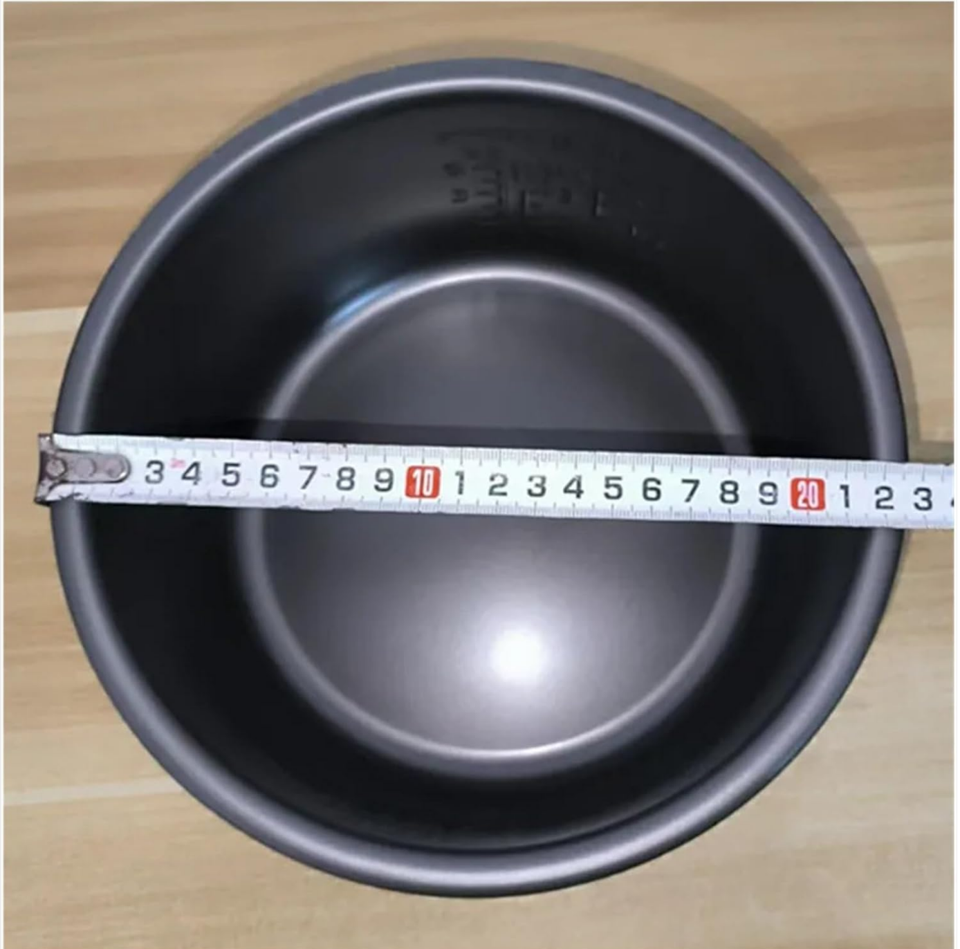
Figure 7.1: Top-down view of the inner bowl with a measuring tape, indicating an approximate diameter of 20cm (8 inches).
