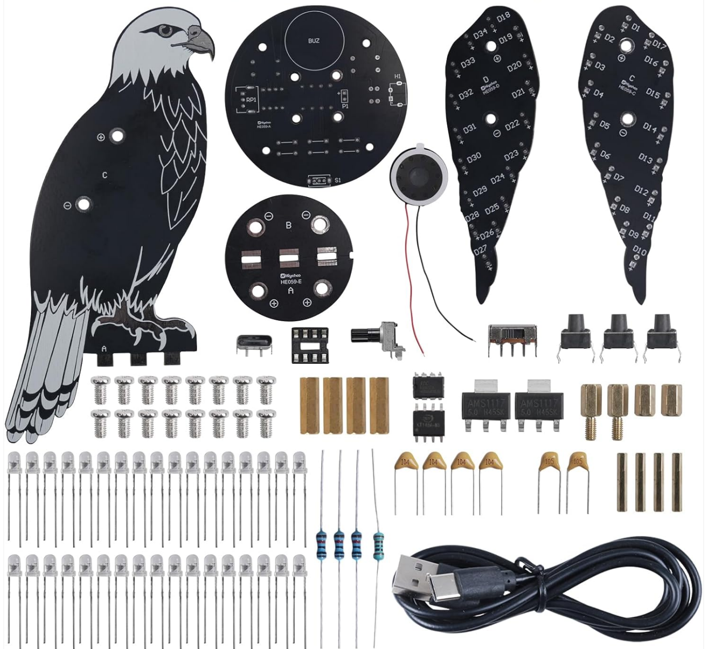
Image: All components of the kit, including the eagle PCB, main board, speaker, LEDs, resistors, capacitors, buttons, and USB cable.
