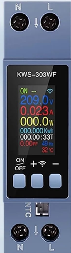
Figure 4: View of the 0.96-inch TFT color screen, showing clear display of voltage, current, power, energy, timing, power factor, frequency, and temperature. (Image shows KWS-303WF, KWS-303L, and KWS-303 variants)
