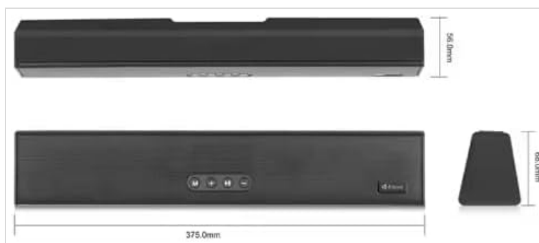
Figure 3: Dimensions of the Kisonli LED-805 Bluetooth Music Speaker.
