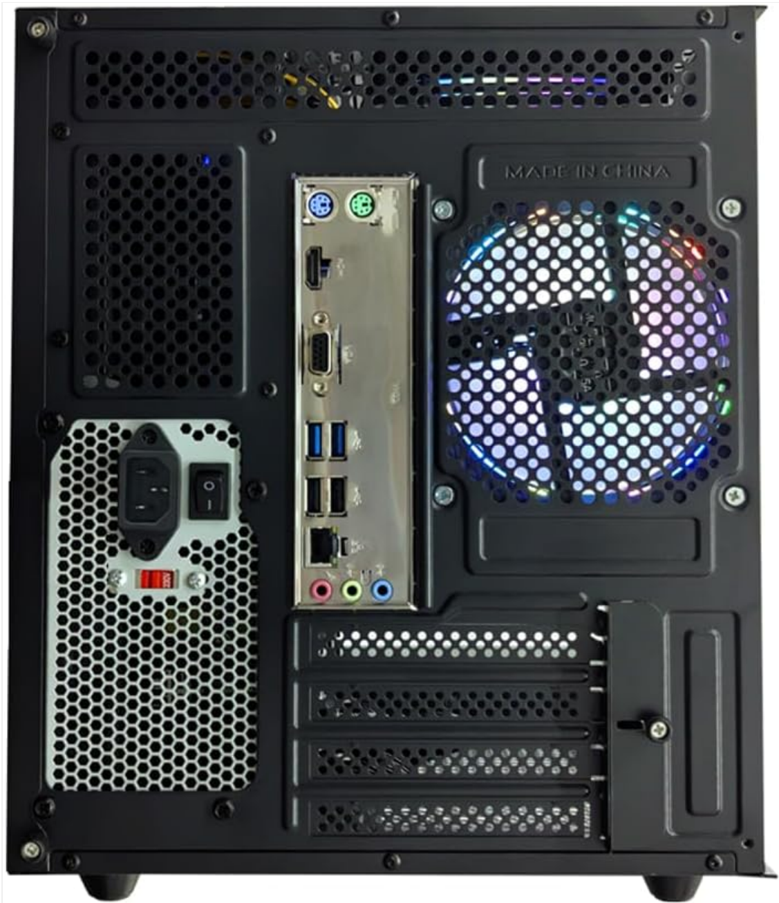
Image 2: Rear panel of the PC, illustrating the available USB, HDMI, VGA, and audio ports for connecting peripherals.
