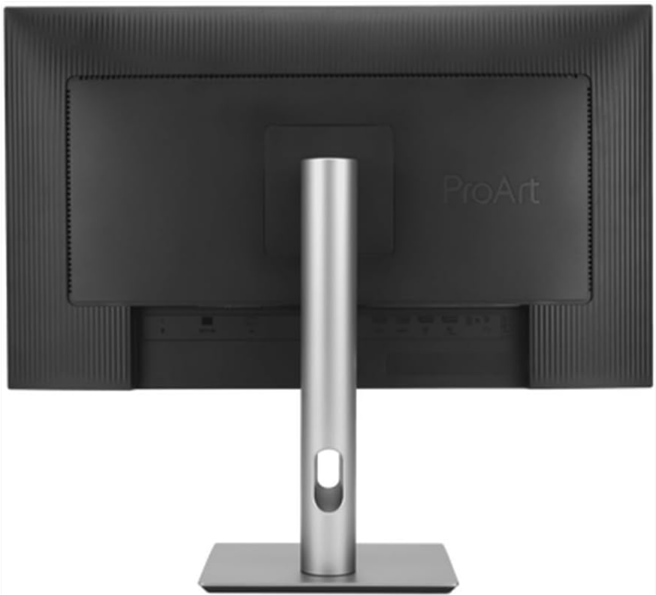
Figure 2.1: Rear view illustrating the connectivity ports including USB-C, HDMI, and DisplayPort.
