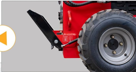
Figure 5.3: Foldable foot pedal and bucket detail.
