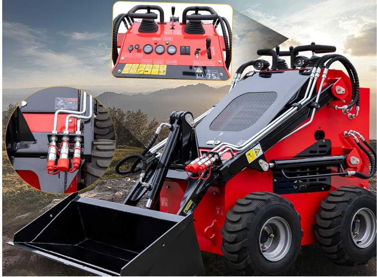
Figure 4.2: Hydraulic connections for multi-attachment compatibility.
