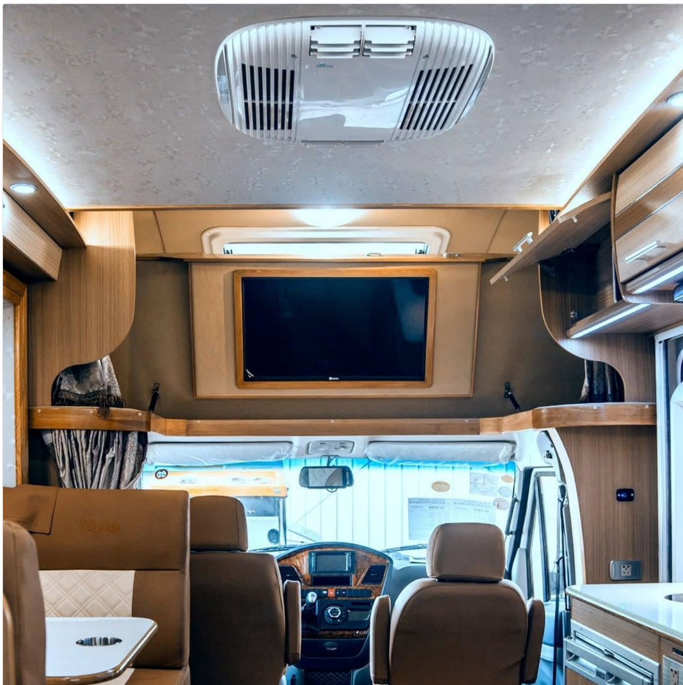
Figure 3: The indoor air distribution box of the Belaire H2000K, seamlessly integrated into the ceiling of a motorhome, providing efficient air circulation.
