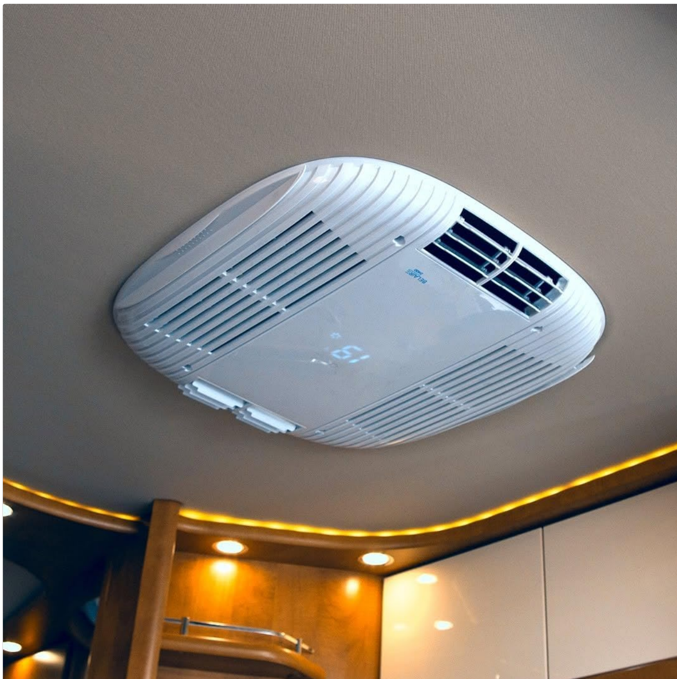
Figure 4: A close-up view of the Belaire H2000K's indoor unit, highlighting the integrated digital display that shows the set temperature.
