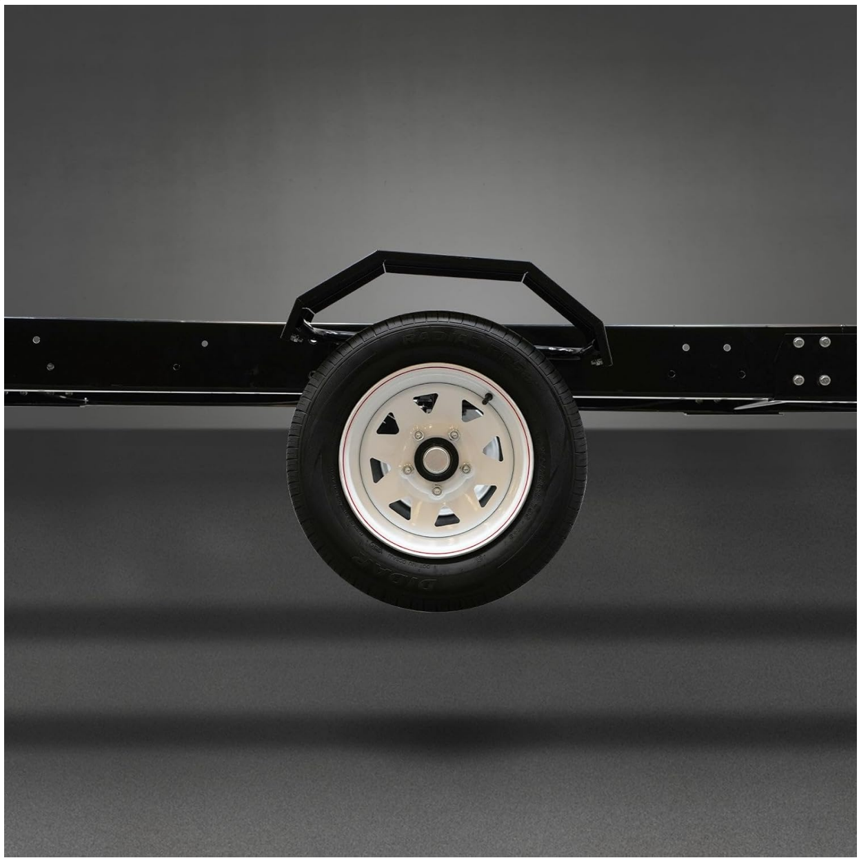
Image 3.2: A close-up view of one of the 6.5/2.8in-R13 DOT approved tires.
