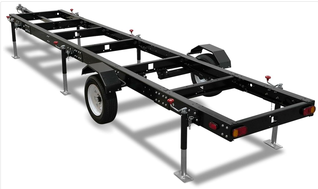
Image 2.2: The complete sub-frame and trailer assembly, showcasing the wheels and leveling jacks.
