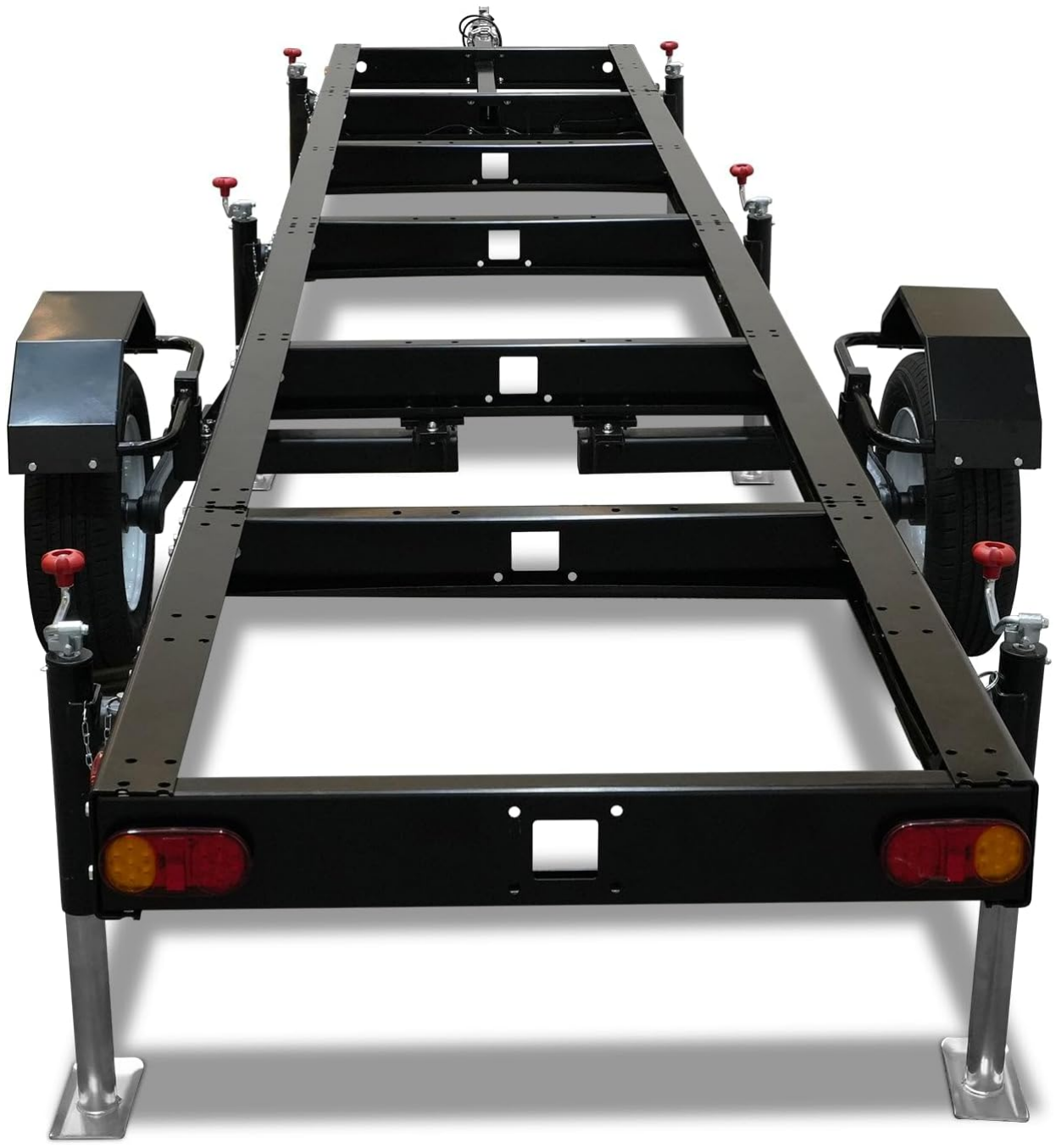
Image 4.1: Rear view of the sub-frame, highlighting the LED stop, turn, and tail lights, and the rear leveling jacks.
