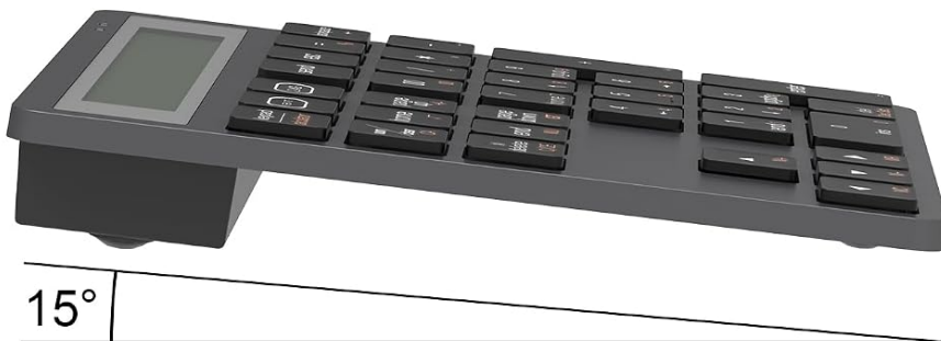
Image 4.3: The ergonomic tilt and quiet scissor-switch keys provide a comfortable typing experience.
