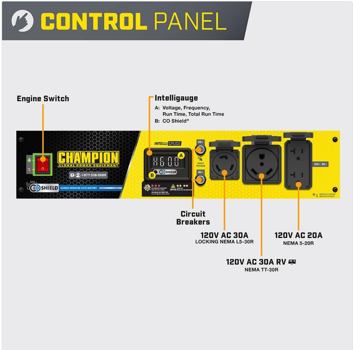
Image: The control panel features an engine switch, Intelligauge display (voltage, frequency, run time, CO Shield status), circuit breakers, 120V AC 30A locking outlet (L5-30R), 120V AC 30A RV outlet (TT-30R), and 120V AC 20A household duplex outlet (5-20R).
