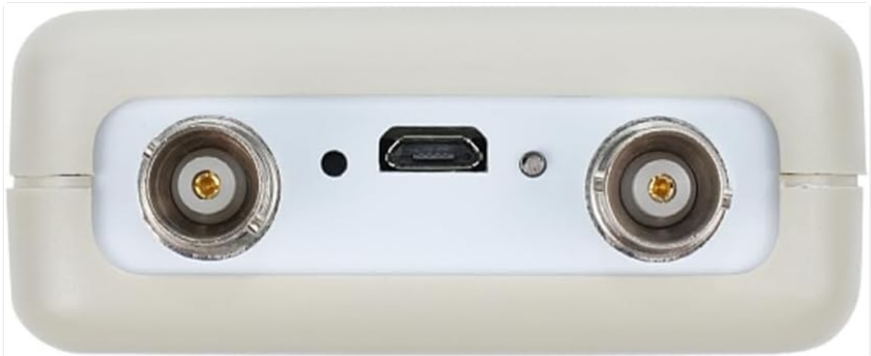
Figure 2: Rear view of the Fosc21C1 oscilloscope, highlighting the Micro-USB port in the center and the two BNC input connectors on either side.
