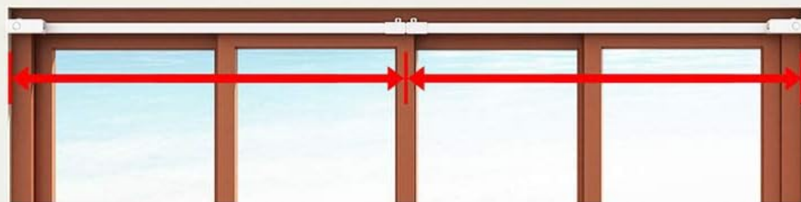
Figure 5.1: Measurement Guide. Measure the dimensions of your door or window frame according to the diagram. If the required rail length exceeds 2 meters or if there are more than two windows, consult for special solutions.
