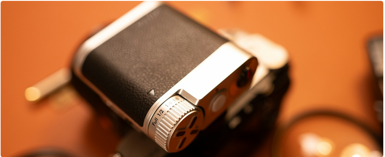
Figure 6: Adjusting the flash power using the dial.
