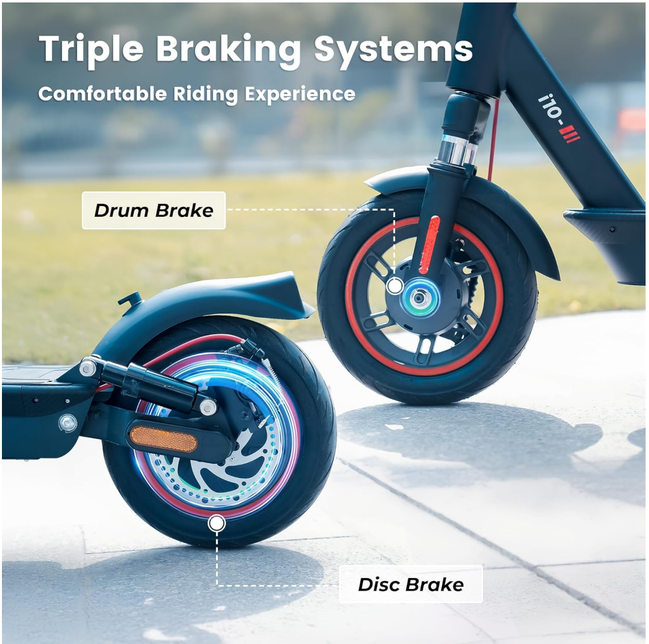
Image: Close-up view of the iScooter i10's triple braking system, highlighting the drum brake and disc brake.
