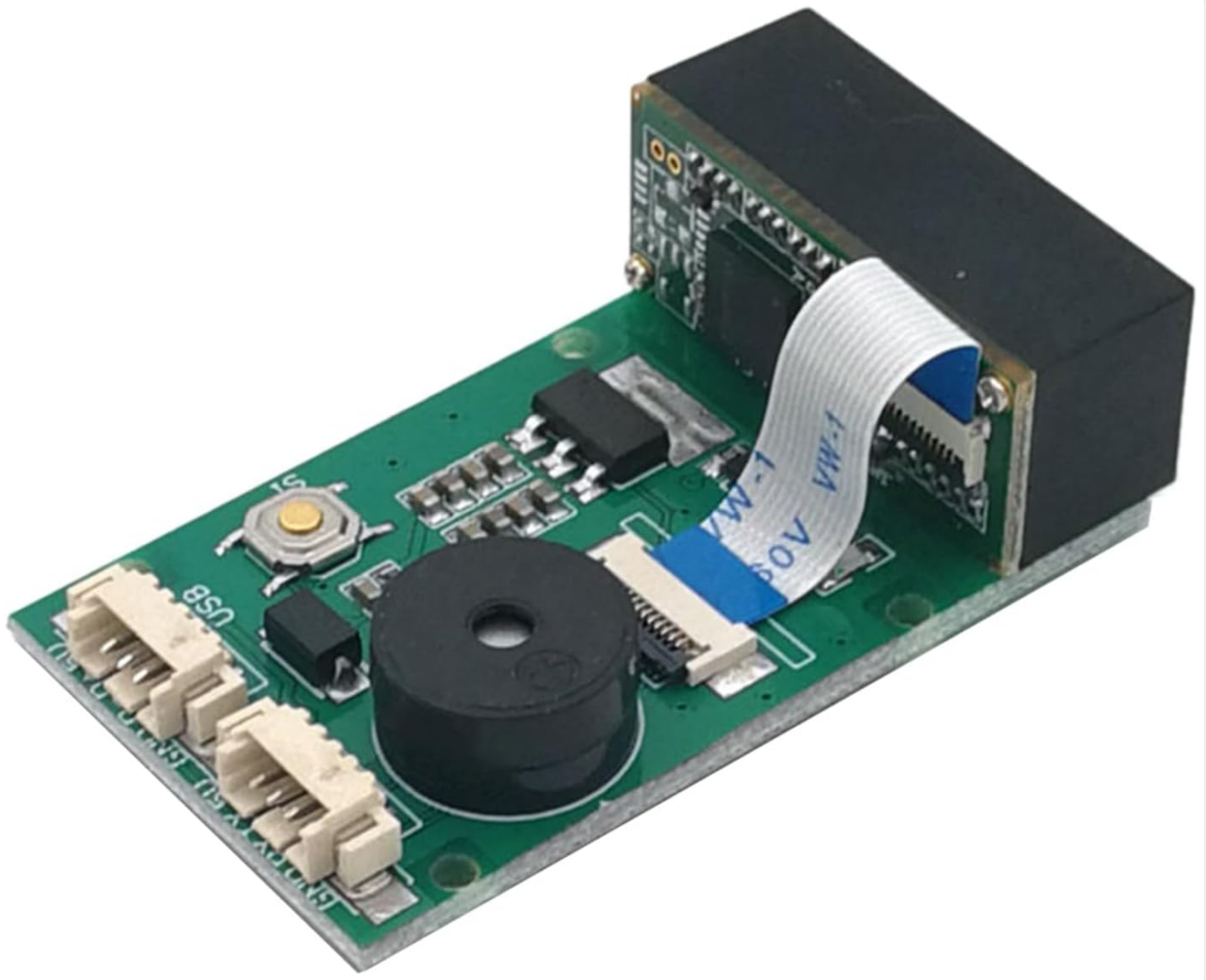
Image: Side view of the GM67 module, showing the flexible ribbon cable connecting the scanner head to the main circuit board.
