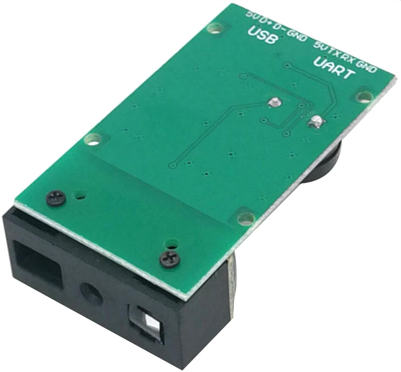
Image: Bottom view of the GM67 module, highlighting the USB and UART connection pads for integration.
